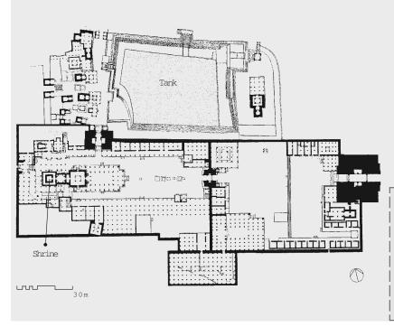
Fig. 7.21 A plan of the Virupaksha temple Most of the square structures are shrines. The two major gateways are shaded in black. Each tiny dot represents a pillar. Rows of pillars arranged in lines within a square or rectangular frame appear to demarcate major halls, pavilions and corridors.
